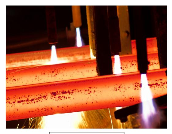
Fig. 7 cutting by gas torches
