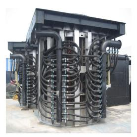
Medium Frequency Induction Melting Furnace
